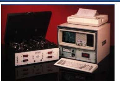
The MDC Model 8512 DuoChuck Integrated Hot Chuck System is the first hot chuck system designed by a C-V plotter company for use exclusively with computerized C-V plotters. Several unique features of this hot chuck system enable faster and more efficient mobile ion measurements than have been previously possible.
