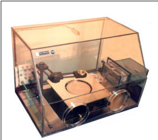
MDC Glove Box for Cu Diffusion Testing Model DG-8 includes airlock for transfer of samples, a hot chuck for temperature stress, video microscope stand, and feedthrough panel for multiplexer and instrument connections.
