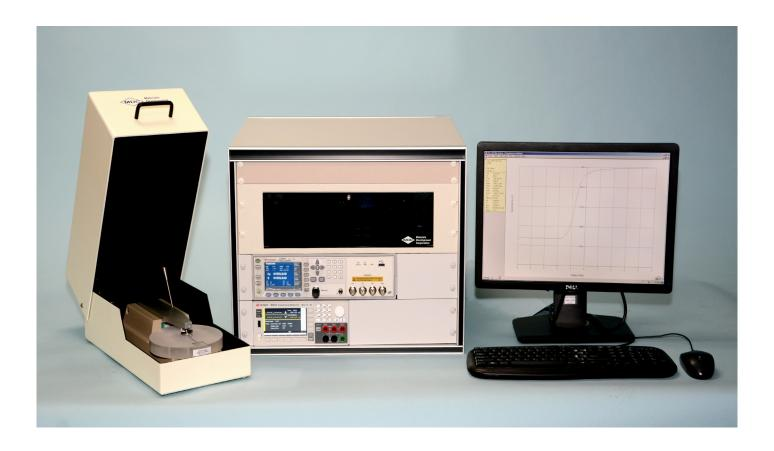
Whether you require a simple C-V plotter to measure mobile ion contamination or an advanced system to measure multi-frequency C-V, I-V, TVS, or gate oxide integrity, Materials Development Corporation has a computerized system for you. And that system comes complete with all necessary hardware and the most versatile Windows software available.
